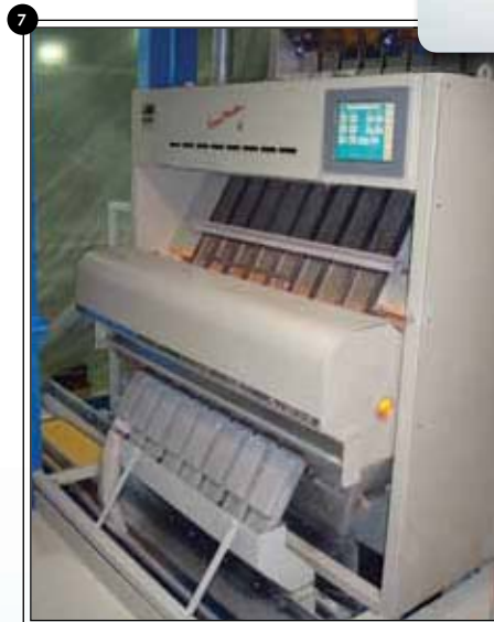
Dahlman's Scan Master II Color Sorter uses infrared cameras to inspect every kernel of seed as it passes through. Lighter kernels and those with defects smaller than .3mm are removed by individual air bursts. The rejected seed is removed from the conditioning line and the accepted seed moves on to treating. The color sorter typically removes about 1-3% of the seed that was passed by the gravity tables. For you that means better quality in every bag.
